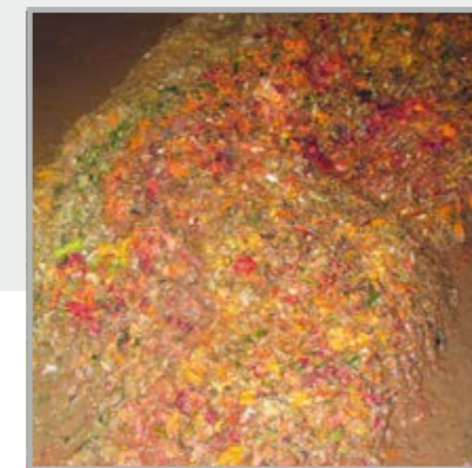
Substrate of the biomass after the pressing process of the EKO 1060 PP
