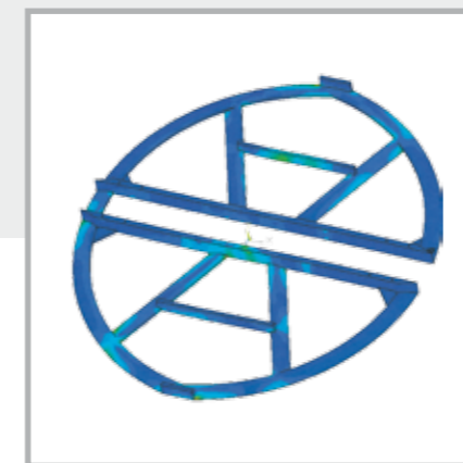
Finite element analysis for the sliding frame
