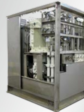
Hydraulic power pack HA 90 S with PCF (Pressure Constant Flow) for pulsation free transportation
