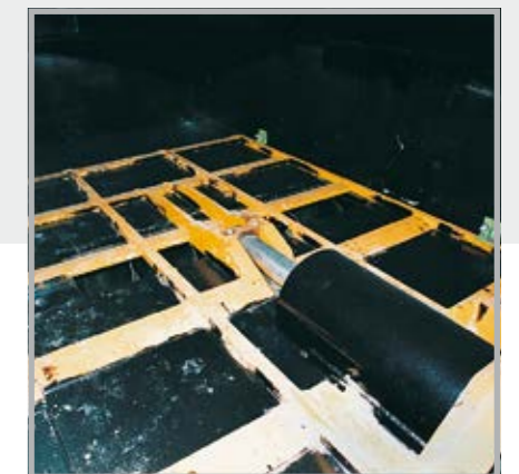
PDL rectangular discharge sliding frame
